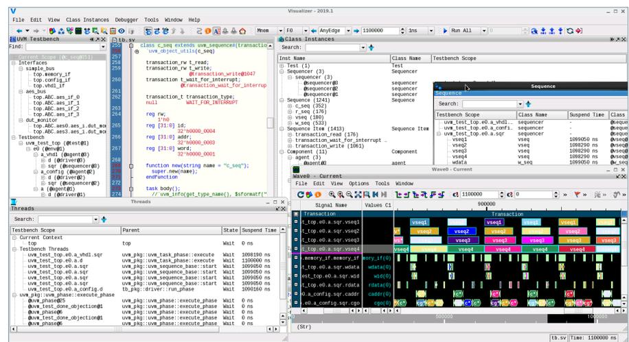
Visualizer's single environment for class-based testbench and RTL DUT debug.
